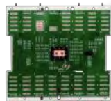
Aries- \gamma \Sigma \Delta Wafer-Sort Probe Card
